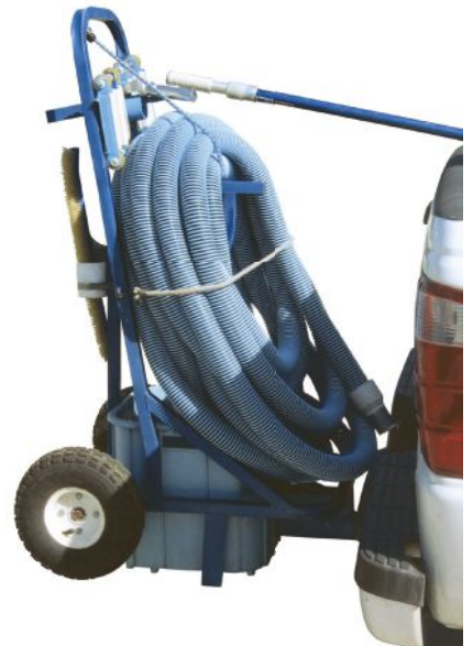
Upwardly mobile: A pool cart, stocked with essential tools, can be towed behind a tech's truck and then wheeled directly to the job site.
