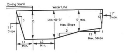
Note: Minimum depth of five feet must be maintained when a wall terminates pool area opposite diving boards. Otherwise, the specified shallow area floor slope may be used to shallow end.
